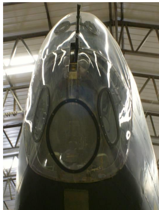
Figure 2 Bomb aimer's position in the nose of a Halifax MkIII
